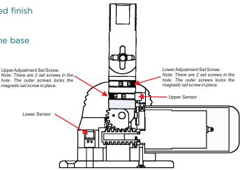
Adjustments to the arm position need to be done slowly 1/4 turn at a time. It is best practice to use an amp meter to determine when the sensor switch disables motor power. Failure to do this could result in motor failure.
